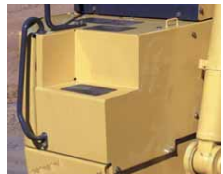
Steps with no-skid sheet provide anti-slip footing for maintenance
