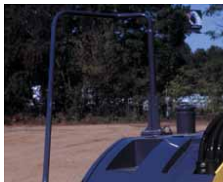
Large handrail is installed for getting on/off machine safely
